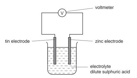
(i) Predict how the voltage of the cell would change if the tin electrode was replaced with a silver one.
